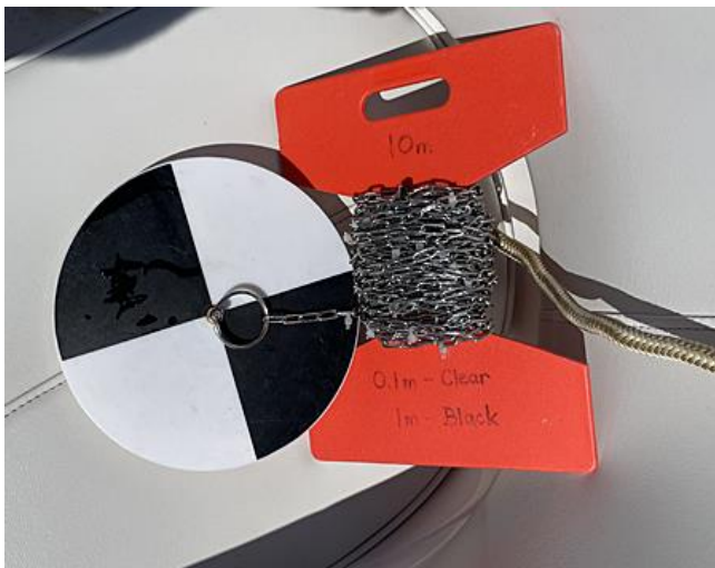
A Sechi Disk, used to measure water clarity. The depth of the water is recorded at the point where one is unable to differentiate between the black and white areas of the disk.
