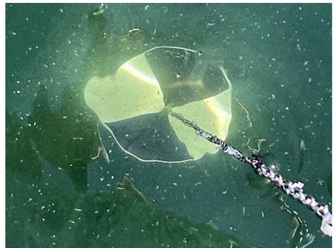
A Sechi Disk, used to measure water clarity. The depth of the water is recorded at the point where one is unable to differentiate between the black and white areas of the disk.
